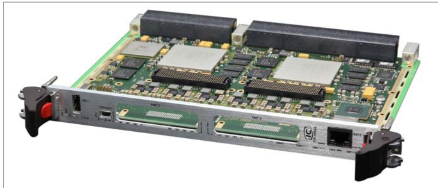
Figure 1 | IC-FEP-VPX6b featuring two Virtex-7 FPGAs.
