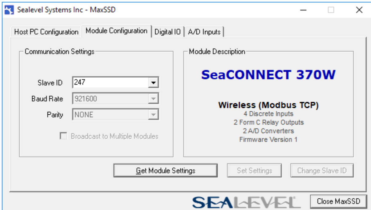
Figure 33: MaxSSD window showing Module Configuration and I/O Tabs
